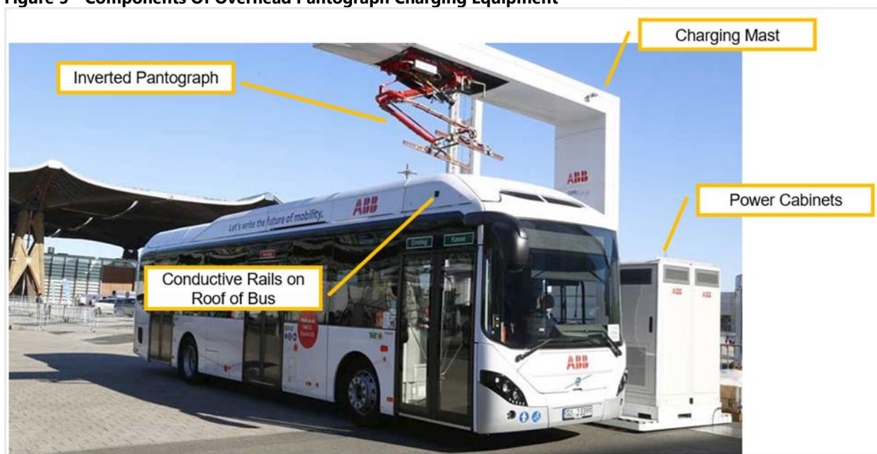
Figure 5 - Components Of Overhead Pantograph Charging Equipment
